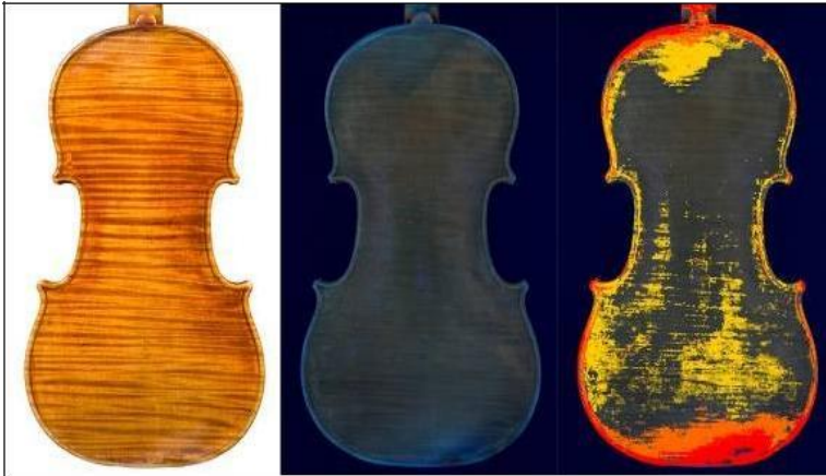
Figure 1: Example of the application on the back of Antonio Stradivari Cremonese (1715). From left to right: visible, UV fluorescence, final result.
