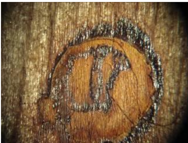
Figure 1: A wooden mock-up stained with iron corrosion products
