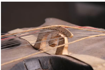
Figure 1: Bridge of bone on an Indian stringed instrument deformed and cracked by the tension of the strings (Esray.) RMT 67/83, Ringve Music Museum.
