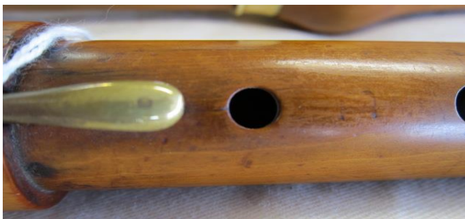
Figure 1. 4935 Bb 5 J.F Simiot, Lyon, circa 1810 Boxwood. Split initiating at L1. © C. Young
