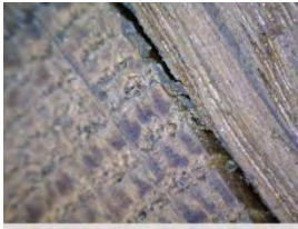
Quercus sp. - growth ring boundaries distinct, wood ring-porous, vessels in dendritic pattern, Ray height > 1 mm. "Mother" muselaar wrestplank.
