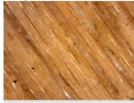
Populus sp. - Simple perforation plates, intervessel pits alternate, rays exclusively uniseriate, all ray cells procumbent. 5' muselaar keylever n°45.
