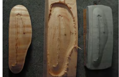
Figure 8: Cello ribs through patch: at right the silicon replica, centre and left wood patches (courtesy Simeoni)
