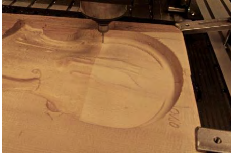
Figure 7: CNC vertical milling of a violin top patch
