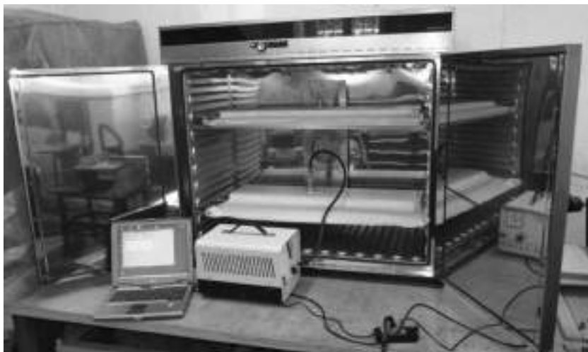
Fig.3 Sealed wood packages in a lab oven during the vacuum procedure.
