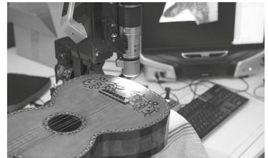
Fig.2 Microscopic investigation of a historical guitar (Beau, build in 1844. MDMB 456) with the digitized image analysis system.
