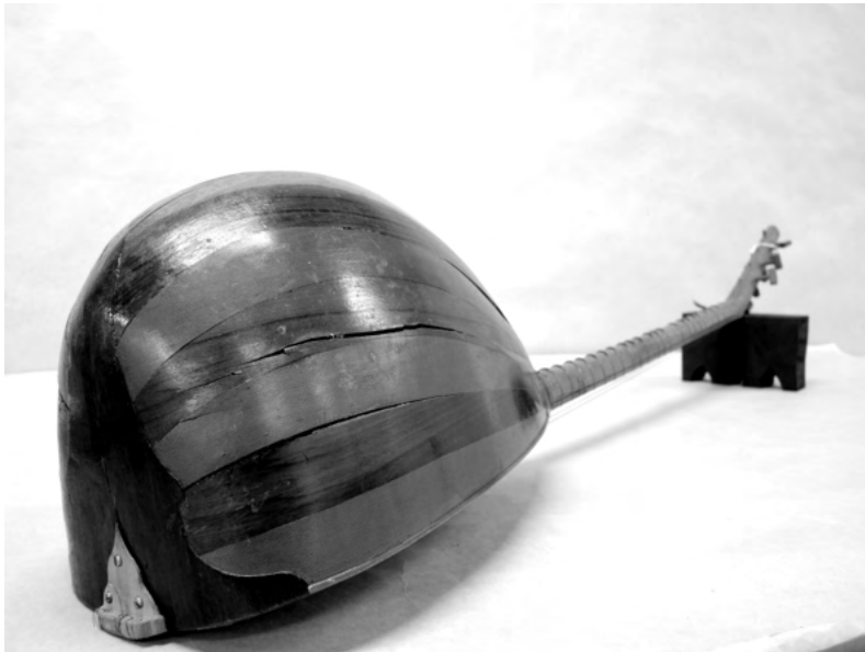
Figure 5: Sound box of a long-neck lute from Turkey made of glued ribs. Some of them are cracked and disassembled.
