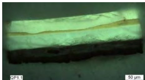
Figure 6: Microscopic photograph of sample from a similar Erard harp (serial No. 3643), showing a similar layer structure as DMO 16147 (photograph © Franziska Bühl).
