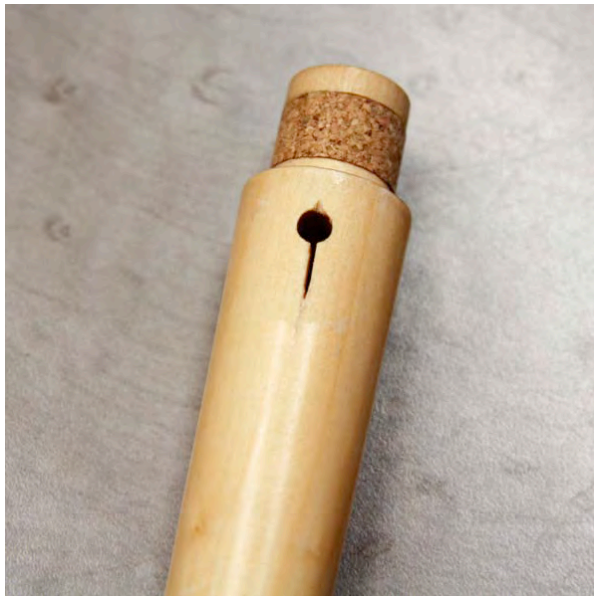
Figure 2: The artificial crack
