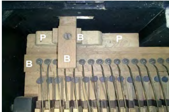
Figure 5: Inner parts of the instrument, where beech (B) and poplar (P) were used
