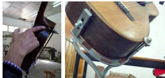
Figure 5: The tripodium fits the drill holes at the bottom and neck joint heel
