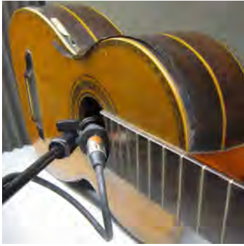
Figure 2: Setup for the acoustic impulse response measurement.
