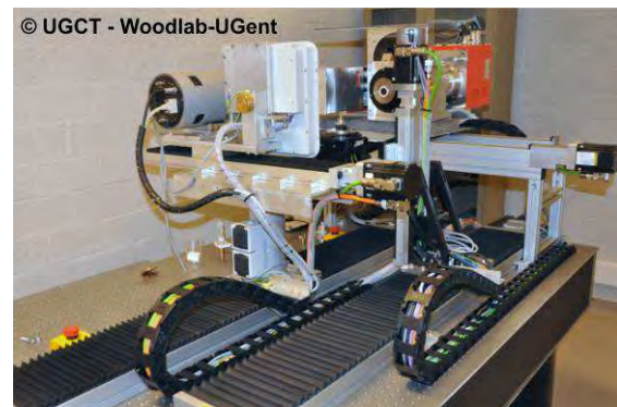
Figure 1: Nanowood X-ray CT scanner @ Woodlab-UGent.
