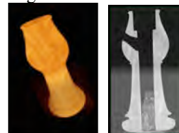
Figure 3, \mu CT surface rendering and tomogram of Cahusac foot joint
