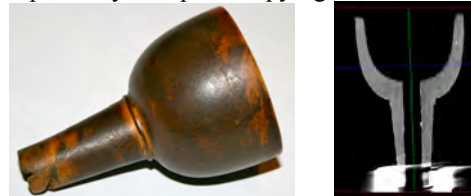
Figure 1, visual and \mu CT views of an ophicleide mouthpiece
