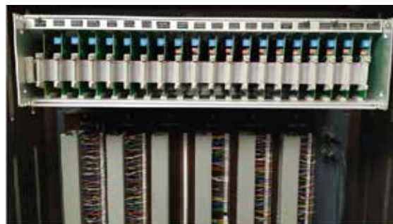
Fig.2: The MIDI-Interface of the theatre organ. Each colored cable is conducting signals from the input and output coming from the ports on the right side and the console. The connected analog-digital-converter is located on the top of the picture.
