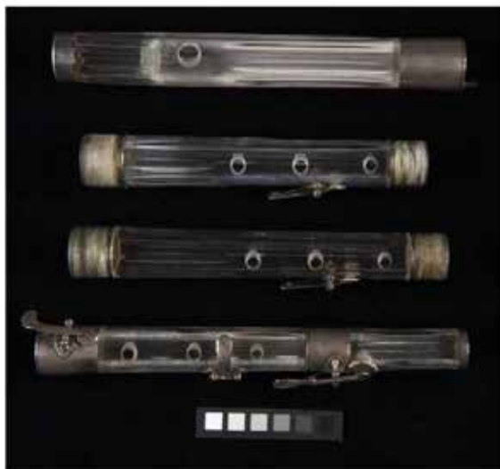
Fig. 4: Normal Light photograph of DCM 475 showing different levels of clarity or opaqueness in joints with similar potash glass compositions. Joints are (top to bottom) the head joint, short upper body joint, long upper body joint, and joined lower body and foot joints. Photo credit: Dana Hemmenway.
