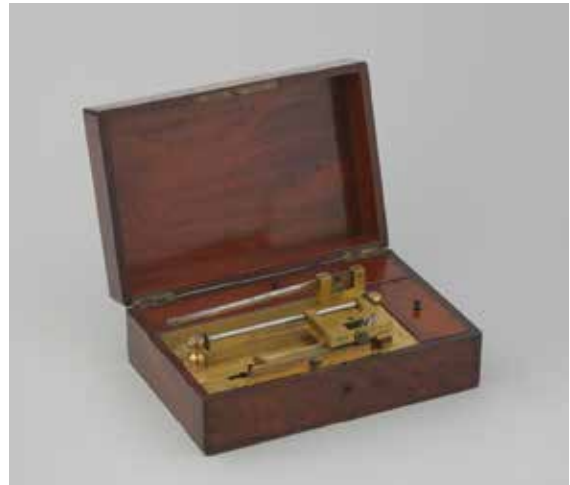
Fig. 5: Reed Gouging Machine by Guillaume Triébert, Paris c. 1850 (Rijksmuseum, inv. BK-2018-6).
